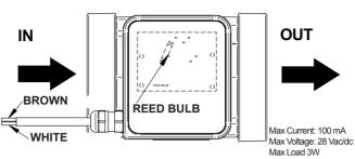
Type output clean contact (open collector)
