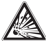
Danger Explosive Material
