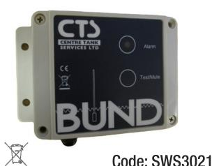
Battery Requirements 9v PP3 (Alkaline Only) **Operating Temps** -20c to +50c **Dimensions** 155 (L) x 95 (H) x 60 (D) mm Colour Light Grey RAL 7035 IP55 IP Rating Nylon Stem, NBR Float, PVC Cable, S/S Clip Float Material S.G 0.70 1 1/2" BSP F Cap Mount Cable Length 5<sub>m</sub>
